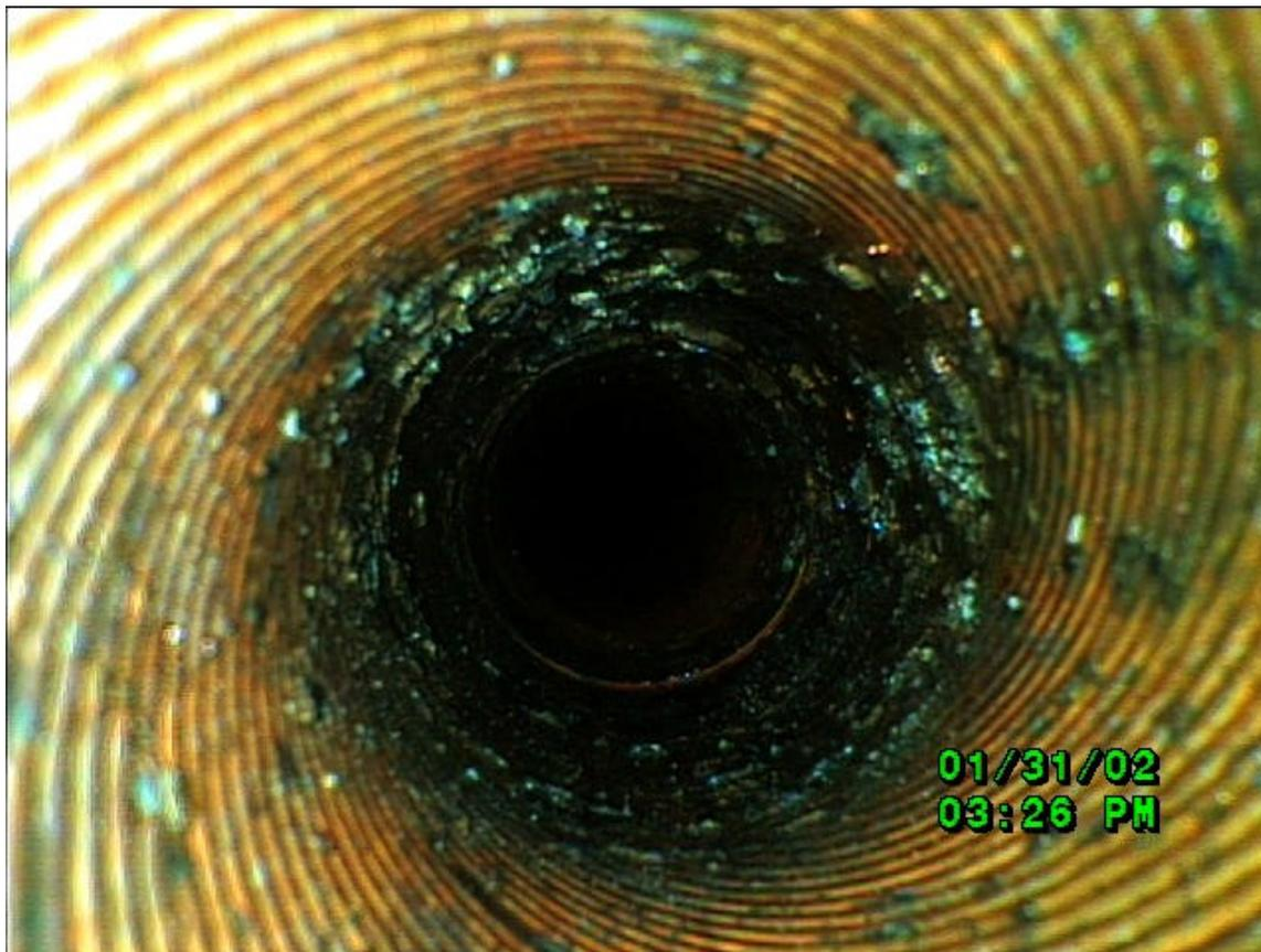
Fiberoptic Scoping reveals severe deposition and corrosion.
