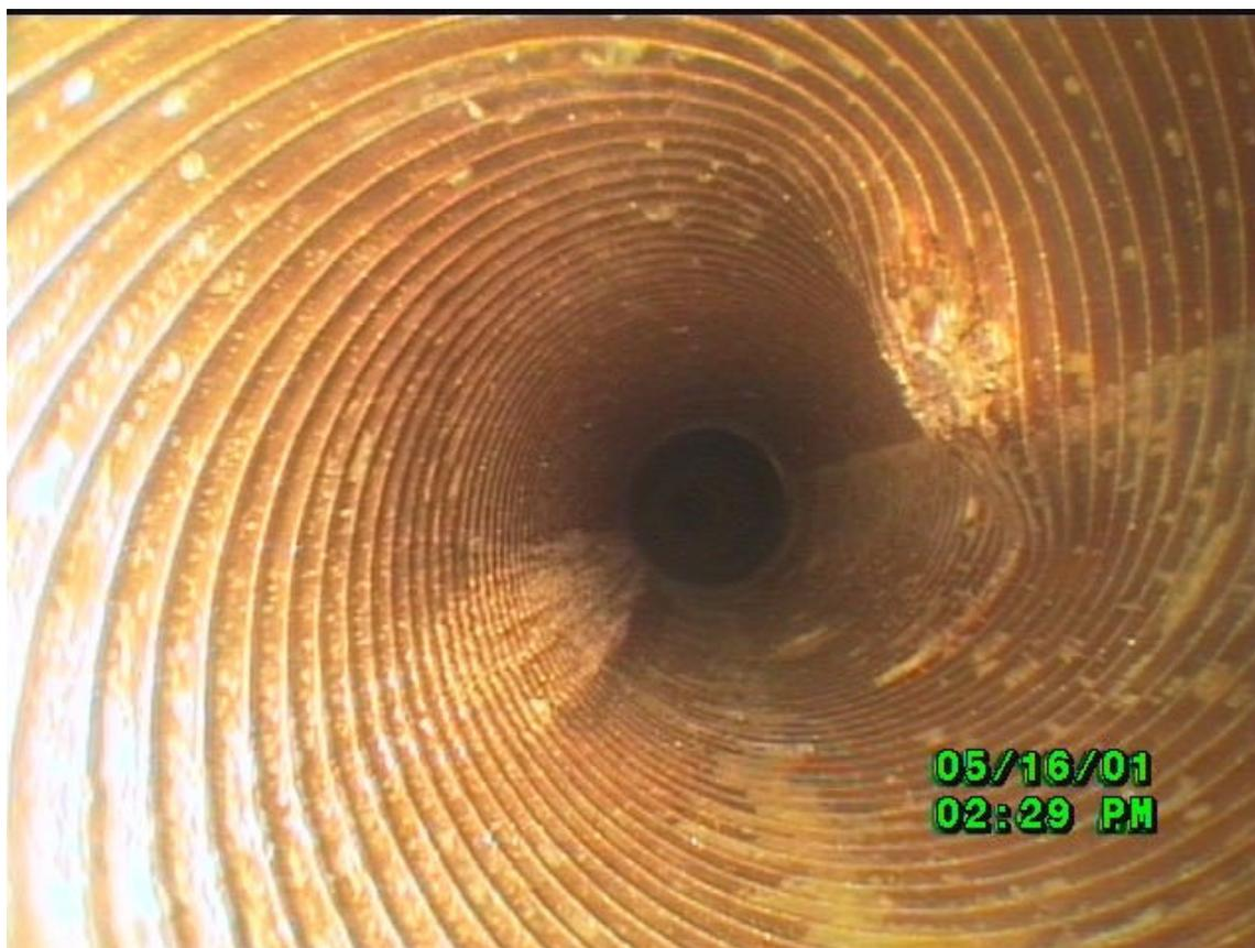
Internal rifling of an enhanced tube is shown with damage to right side of tube.
