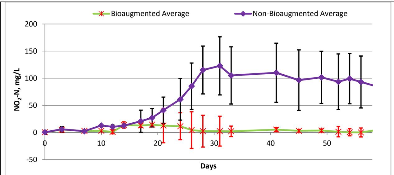
**Figure 3. Bioaugmented digesters showed consistently lower nitrite accumulation. Error bars indicate standard deviation among six replicates**
