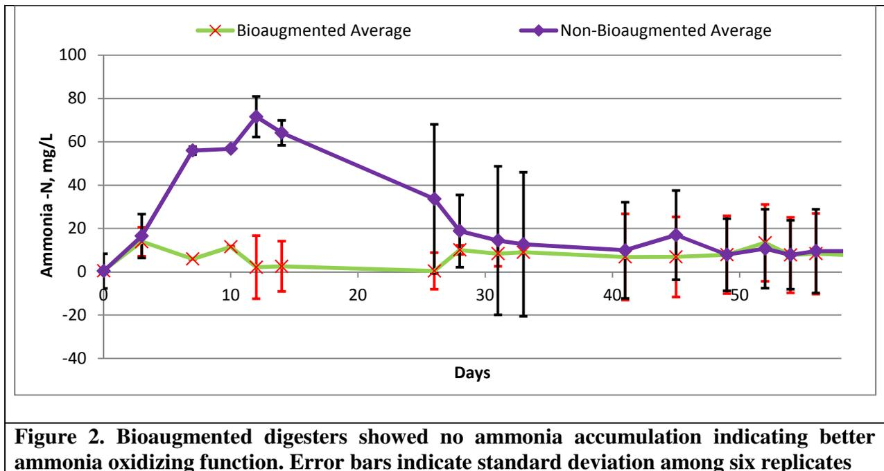
**Figure 2. Bioaugmented digesters showed no ammonia accumulation indicating better ammonia oxidizing function. Error bars indicate standard deviation among six replicates**
