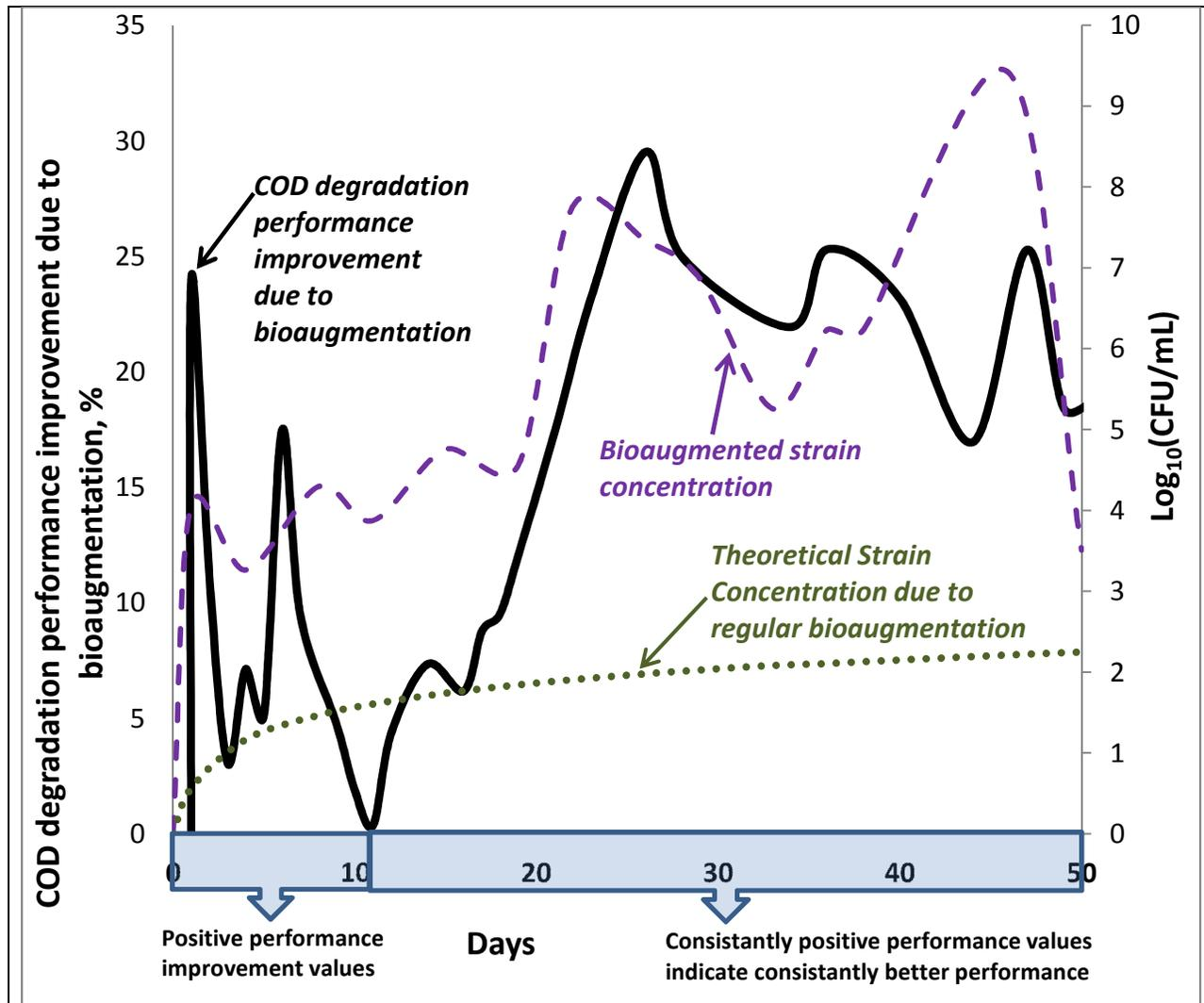
Figure 8. Theoretical total strain concentration (in case of no growth) vs measured total strain concentration and COD removal performance improvement calculated as percent extra COD removed by treated reactors as compared to the untreated reactors
