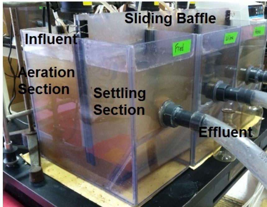
**Figure 1. Eckenfelder type flow-through reactors used for the laboratory bioaugmentation study**
