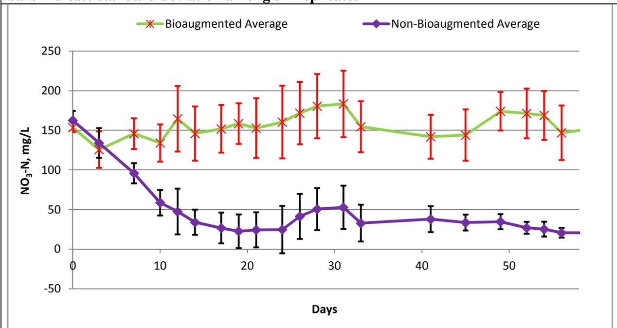
**Figure 4. Bioaugmented digesters showed consistently higher nitrite production indicating better ammonia and nitrite oxidation performance. Error bars indicate standard deviation among six replicates**
