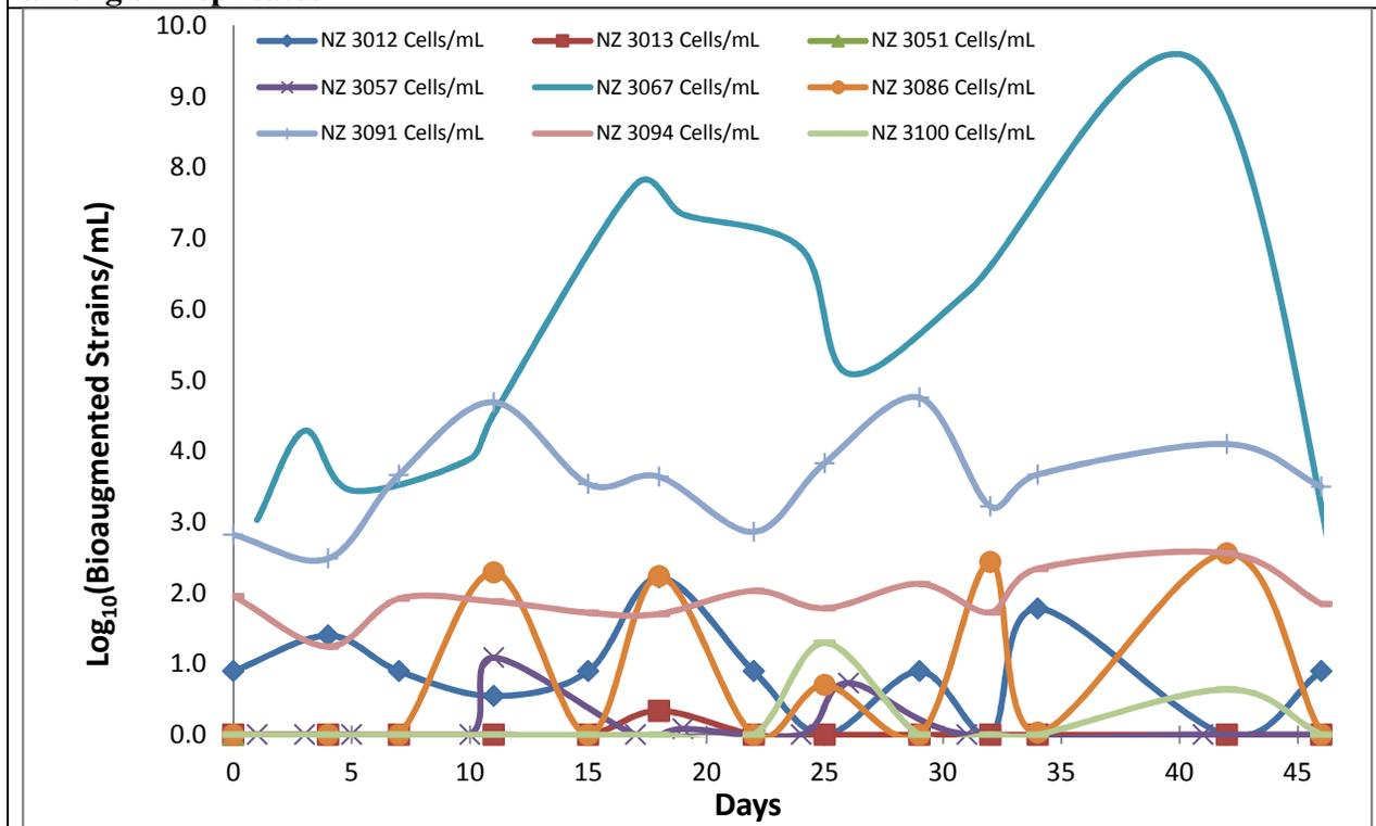
**Figure 7. Actual concentration of the bioaugmented strains in the mixed liquor measured by qPCR. Concentrations above the dosing line indicate growth**
