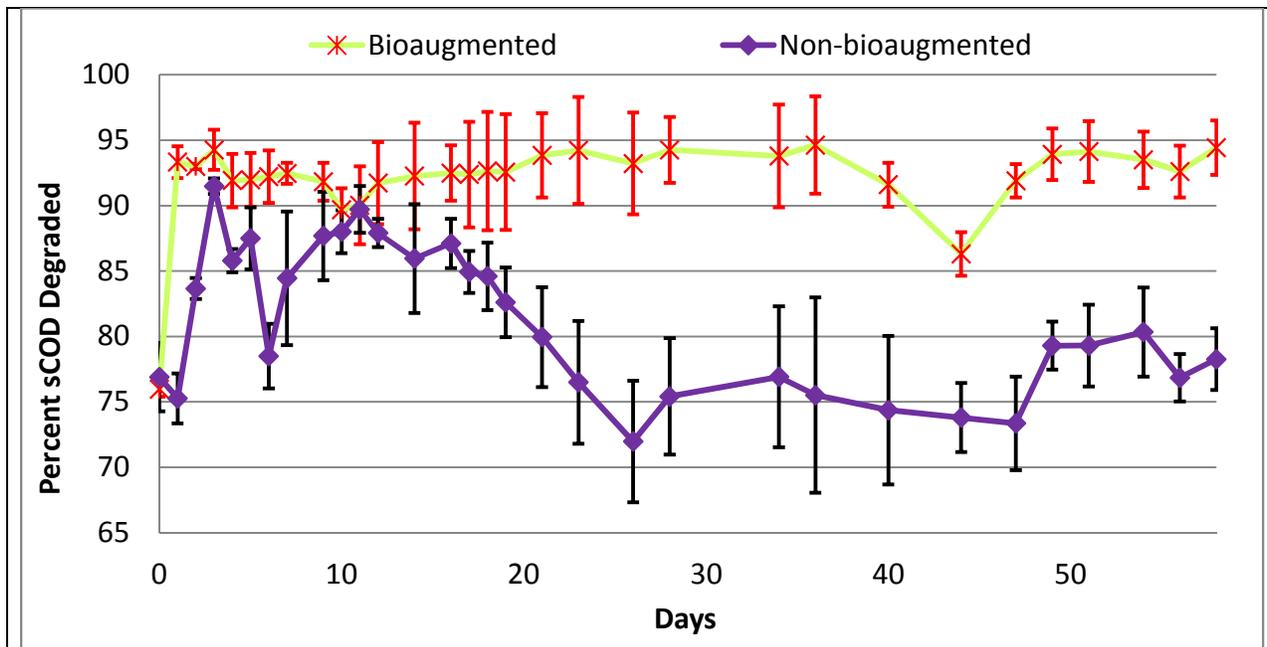
**Figure 6. Bioaugmented digesters showed consistently better and stable performance as compared to the non-bioaugmented digesters. Error bars indicate standard deviation among six replicates**
